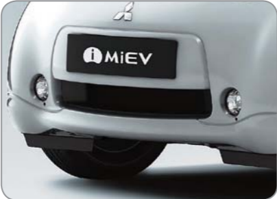
Front fog lamps with Daytime Running Lights
